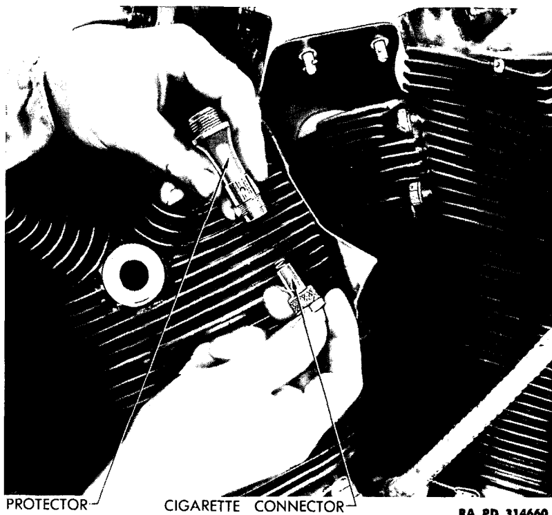
Figure 40 — Installing Protector on Front Spark Plug Cigarette Connector
