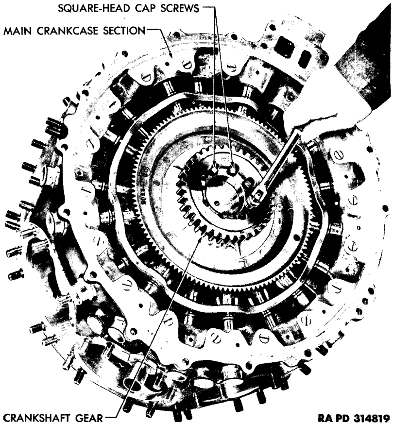
Figure 210 – Tightening Crankshaft Gear Retaining Screws
