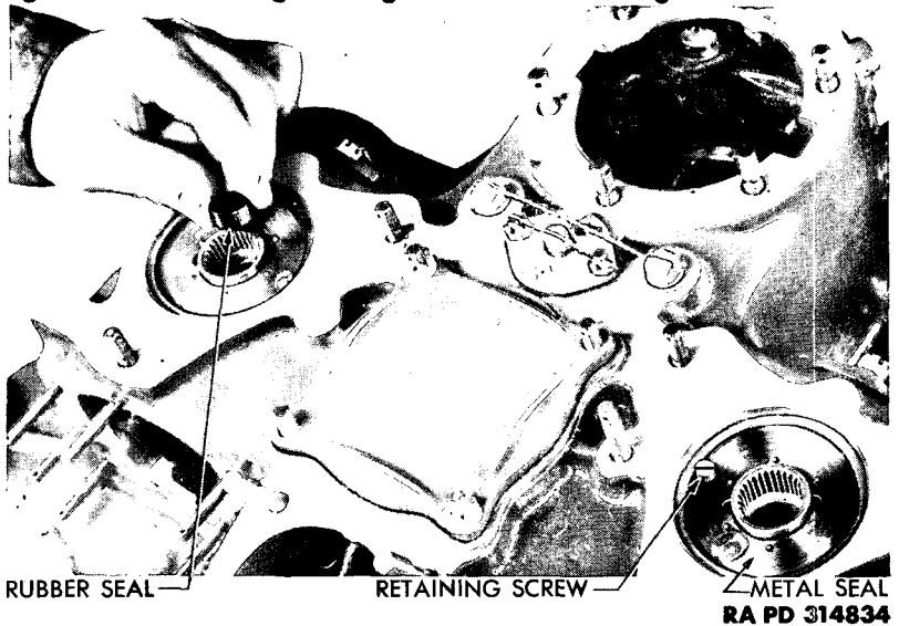
Figure 199 — Placing Rubber Seal in End of Accessory Drive Shaft
